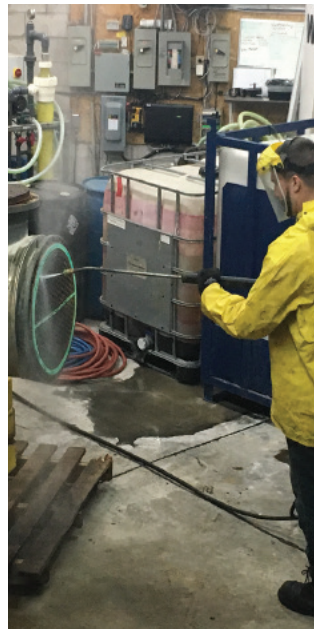
PRESSURE WASHING, CHEMICAL CLEANING
